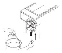
Figure N Clean Valve Body
